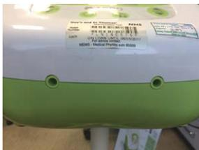
Insert the expressing kit tube into one of the holes on the front of the pump. If double pumping, use two kits and insert one into each hole.
