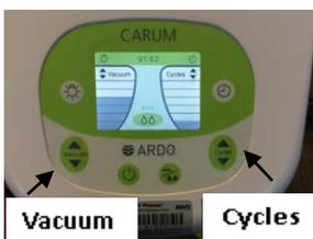
In expression mode use the down arrow marked cycles to turn the cycles down low. Use the up arrow marked vacuum to increase the suction to a comfortable level for you. In this mode the top line is green. When you have completed expressing from one breast, switch the pump off and move to the other breast and start again.
