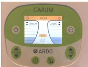
The pump will start in 'stimulation' mode. The top line of the screen is orange in this mode. The cycles will be quite fast but also gentle. This will run for two minutes. It will then automatically switch to 'expression' mode.
